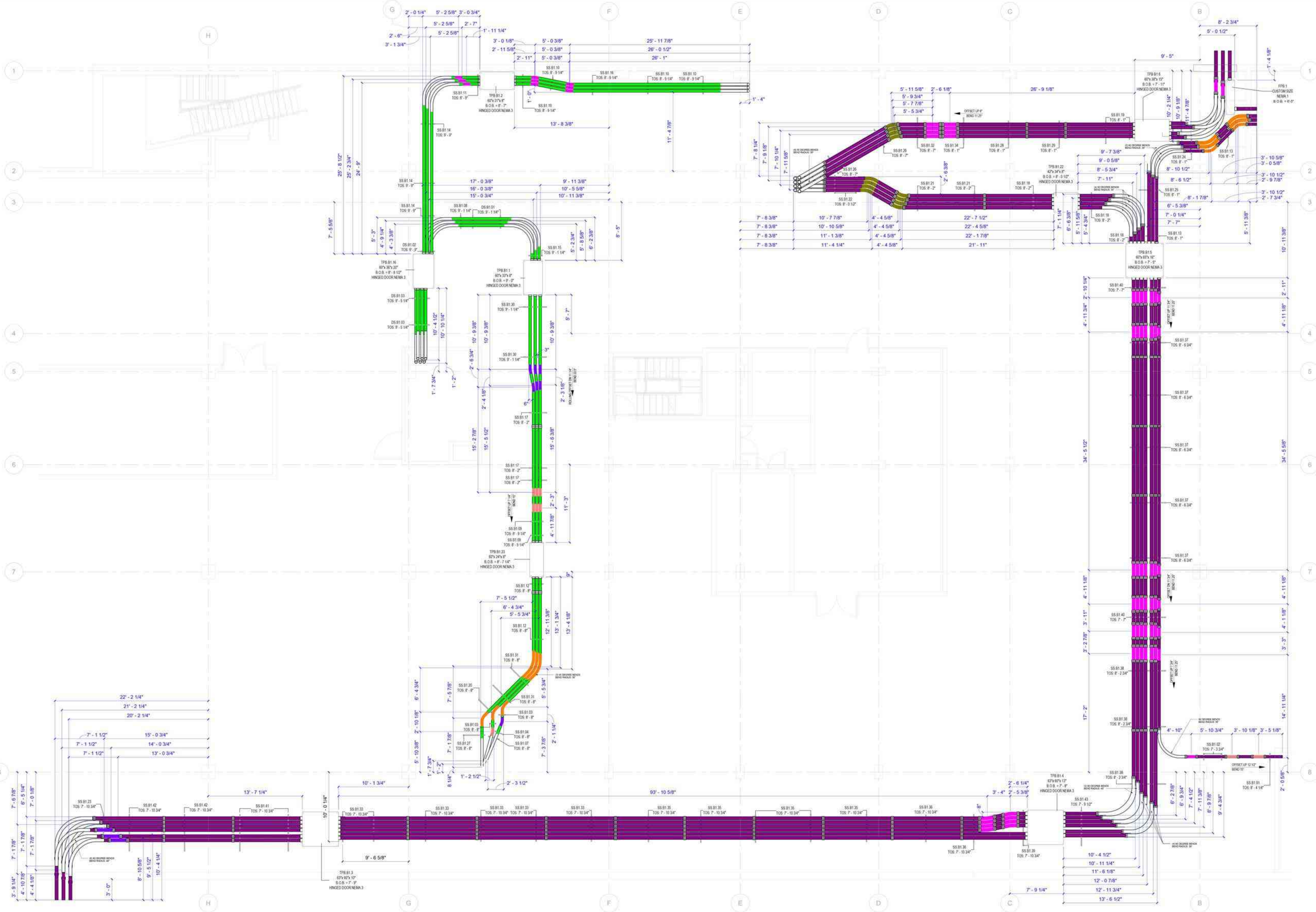
1 TEL/DA/FA CONDUIT LAYOUT LEVEL B1 3/16" = 1'-0"
